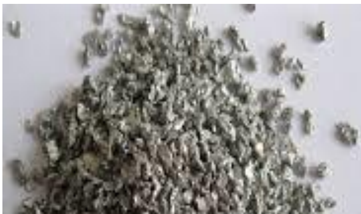
Figure 1 – Microparticles of alloy AK12MMgN powder waste after regeneration (on plastic plate)
